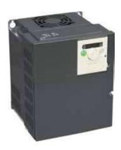
A Variable Frequency Drive (VFD) completely eliminates the large starting inrush current of the compressor by ramping up voltage and frequency in a controlled time period. This allows running on limited dockside power, and also protects the generator from overload.
