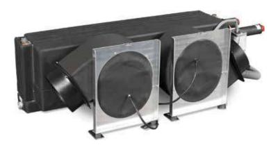
The ABL-HV series of draw-through air handlers for chilled water systems is ideal for installation in height-restrictive spaces. Insulating foam covers the condensate pan, blower housing, shroud, and coil end cover to reduce noise and secondary condensation. The condensate pan also has an antislosh, anti-fungal foam lining. The ABL-HV series is designed to replace the CBLB models.
