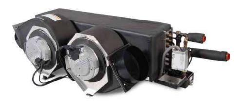
The ABL-DC series of marine draw-through air handlers for chilled water systems is ideal for installation in height-restrictive spaces. Insulating foam covers the condensate pan, blower housing, shroud, and coil end cover to reduce noise and secondary condensation. The condensate pan also has an anti-slosh, anti-fungal foam lining. The ABL-DC series is designed to replace the CBLB models.
