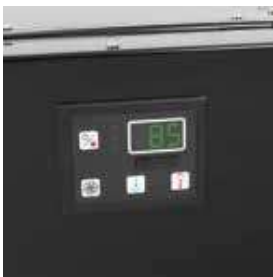
Digital Passport Compact keypad/control with LED read-out is mounted on the unit.
