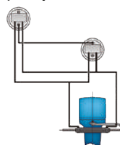
Dual steering position for one engine
